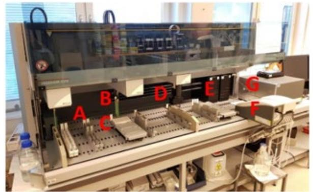
Ready-to-use reagents were put into predefined cups (A) and samples were loaded onto the robot. An 8-channel pipettor (B) was used to transfer sample and reagent material between tubes/cups and the 96-well plate (C). The gripper (D) was used to move the plate into different sections. Each section was specifically dedicated: sample preparation (8-channel pipettor), plate incubation (E), plate washing (F), or UV/Vis spectrophotometry (G).
